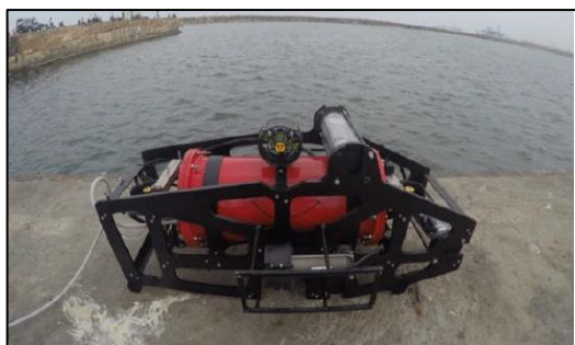
Figure 8-1. An observation class ROV equipped with a high definition video camera, high-intensity LED illumination, and a sonar mapping system.
