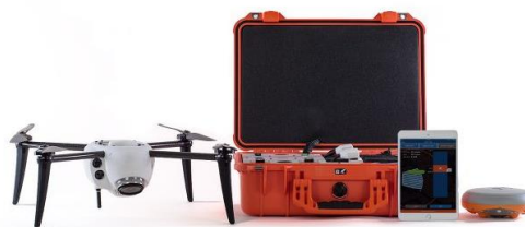
Figure 8-3. Rotary system drones suitable for dam inspection are small and easily transported.
