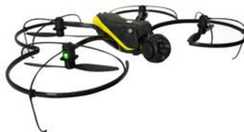
Figure 8-2. In the case of a four-propeller UAV system (quadcopter) such as the one shown, diagonal pairs of propellers spin in opposite directions.
